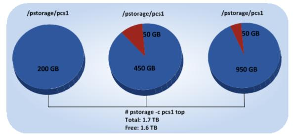
• allocatable 180GB of 200GB is the amount of free disk space that can used for storing data chunks. See **Understanding allocatable disk space** below for details.
