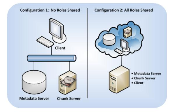
For a Virtuozzo Storage cluster to function, it must have at least one MDS server, one chunk server, and one client. The minimum configuration has two main limitations:
