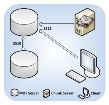
By default, Virtuozzo Storage uses port 2510 for communication between MDS servers and port 2511 for incoming connections from both chunk servers and clients. You can override the default ports when creating MDS servers:
