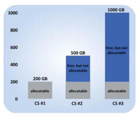
In this example, the available disk space will equal 200 GB, that is, set to the amount of disk space on the smallest chunk server:
