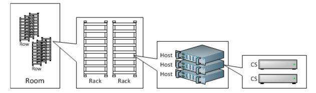
The first 3 topology path components, room.row.rack, can be configured in the /etc/pstorage/location configuration files (for more information, see the man page for pstorage-config-files). The last 2 components, host\_ID.cs\_ID, are generated automatically:
