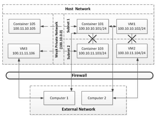
In this example, the private network on the physical server is divided into two subnets: *Subnet 1* and *Subnet 2*. Container 101 and VM1 are connected to Subnet 1, and Container 103 and VM2 are joined to Subnet 2. Container 105 and VM3 do not belong to the private network. Container
