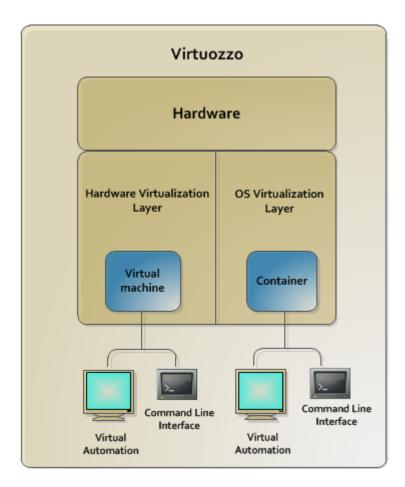
At the base resides server hardware. Next is the Virtuozzo software which is installed directly on the server hardware and does not need any operating system for its functioning. Virtuozzo includes two virtualization layers:
